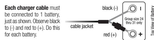
When connecting to an engine start battery only connect the battery bank cable that is LABELED: "FOR ENGINE BATTERY USE THIS BANK CABLE ONLY".
