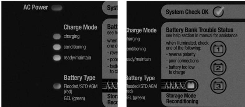
ProSport includes 7 LEDs for operation status and up to 3 battery bank trouble LEDs depending on the model.
