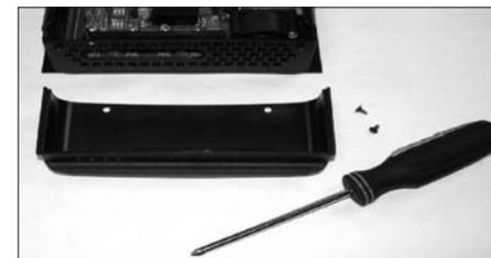
Shown above is the ProTech-i split DC endcap. Please note that this is a two piece end cap. To remove simply unscrew the two self tapping screws on the top of the DC end cap and slide top cap off. This will allow access to the low voltage DC terminals for connections of cables.
