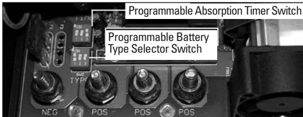
Shown Above - Programmable Absorption and Battery Type Selector Switches. Please refer to page 6 for settings and selections.
