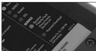
The LED Service indicators provide at a glance assistance in identifying common conditions that with proper attention can prevent damaging the ProTech-i charger and the unnecessary uninstallment of your charger. The two service LED indicators are:
