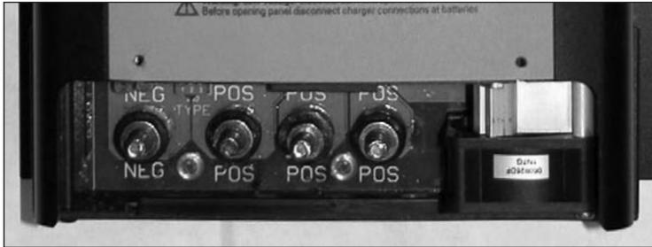
Shown Above: ProTech-i Plus model. The circuit board is clearly marked to identify the polarity of each DC output connection.
