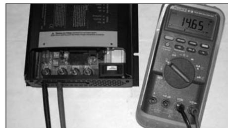
5) If the voltage is 14.6-14.7 keep the charger's AC power on with the DC outputs disconnected from the battery(s). Leave the charger on for approximately one hour, make sure absorption switch is in one hour setting otherwise it could take up to 4 hours or until float mode is observed. The voltage should drop to 13.5 VDC indicating float mode.
